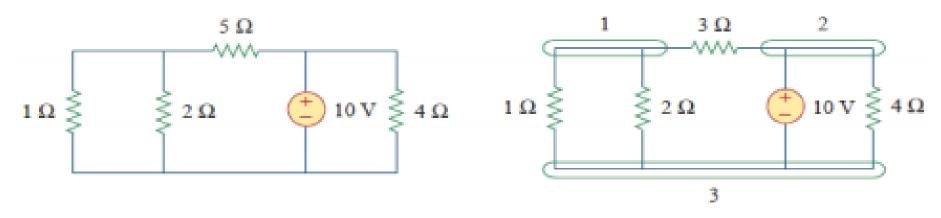
> (b) Five branches and three nodes are identified in Fig. (b). The 1 $\Omega$  and 2 $\Omega$  resistors are in parallel. The 4  $\Omega$  resistor and 10-V source are also in parallel.
