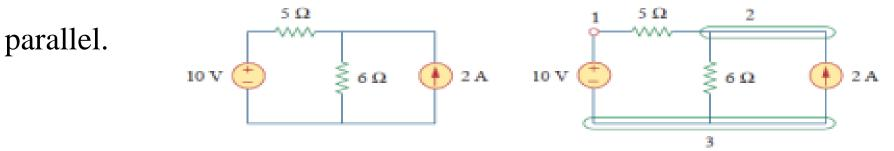
(a) Since there are four elements in the circuit, the circuit has four branches: 10 V, 5  $\Omega$ , 6 $\Omega$ , and 2 A. The circuit has three nodes as identified in Fig. (a). The 5 $\Omega$  resistor is in series with the 10-V voltage source because the same current would flow in both. The 6- resistor is in parallel with the 2-A current source because both are connected to the same nodes 2 and 3.
